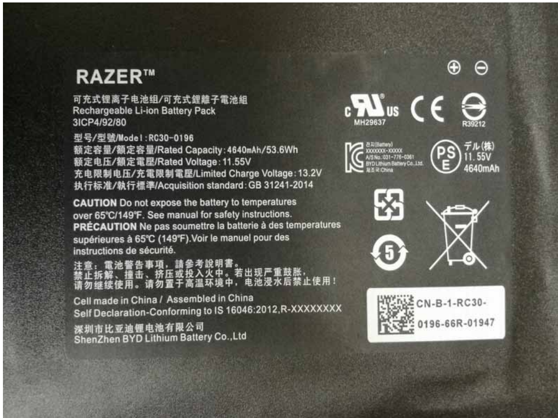
Figure 13 Label of the Battery
