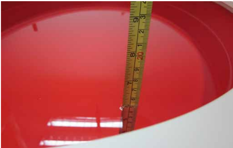
Figure 4.4: Liquid depth in the Flat Phantom
