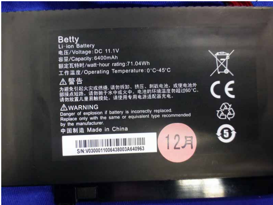
Figure 27 Battery of the EUT
