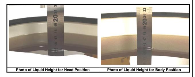
The dielectric properties of the head tissue simulating liquids are defined in IEEE 1528, and KDB 865664 D01 Appendix A. For the body tissue simulating liquids, the dielectric properties are defined in KDB 865664 D01 Appendix A. The dielectric properties of the tissue simulating liquids were verified prior to the SAR evaluation using a dielectric assessment kit and a network analyzer.
