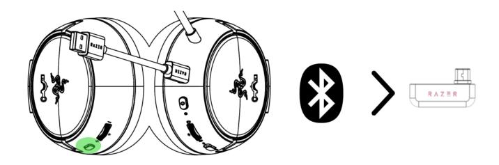
Using Bluetooth as the audio source will reconnect the headset to the last known device. Pairing mode will be activated if no device is found.
