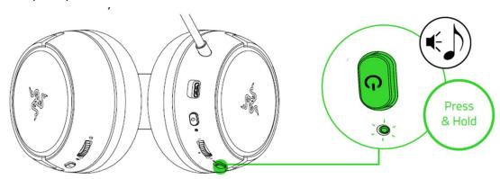
3. Wait until the status indicator briefly becomes static green indicating that the headset is now connected to the Type-C wireless dongle.
