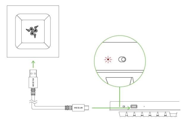
5. Wait for your keyboard to fully charge. The power indicator will light up green to indicate that it has fully charged.
