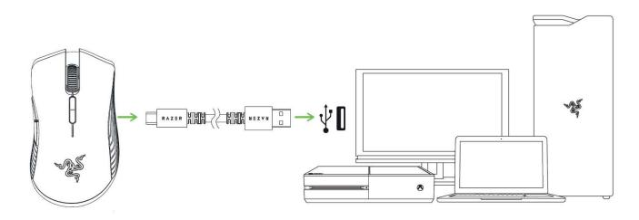
• Note: Connecting the keyboard and/or mouse via wired connection will also individually charge your devices. A USB connection that can supply sufficient power to your device is required. The charging process may be affected if connected to non-powered USB hubs or non-powered USB ports found on certain keyboards and other peripherals. When in doubt, it is recommended to connect these devices directly to the USB ports of either your Xbox One or PC.
