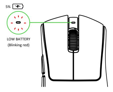
The lighting sequence will repeat until the mouse is drained or connected to a PC via the included cable.
