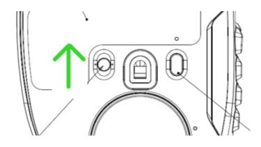
2. Press and hold the scroll wheel, DPI stage up and DPI stage down buttons simultaneously for three seconds to activate pairing mode. The Razer logo will blink twice in repeated intervals to show that the device is in pairing mode.
