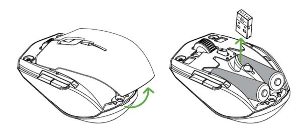
2. Close the top cover and insert the wireless USB dongle into the USB port of your PC.
