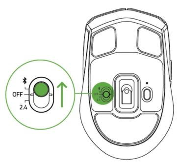
2. Press the pair/switch button to select a slot for your Bluetooth device. You can pair up to 3 Bluetooth devices on your Razer RZ01-0399. The pairing indicator will blink twice in repeated intervals to show that the mouse is in pairing mode.
