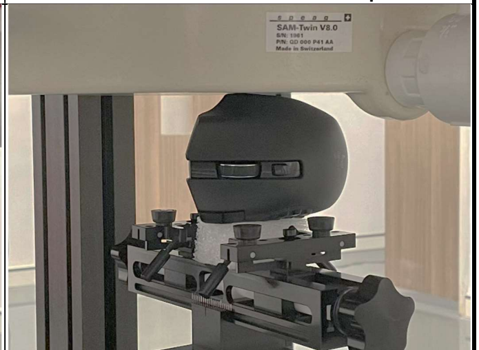
Right Side of EUT with 0 cm Gap
