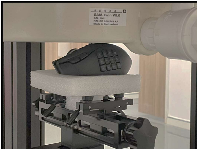
Front Face of EUT with 0 cm Gap
