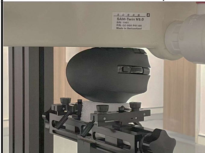
Left Side of EUT with 0 cm Gap
