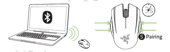
6. When the pairing process is completed, the indicator light will stop blinking. Your Razer Orochi is then ready for use in wireless mode.
