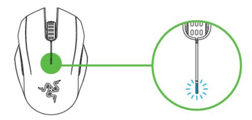
Note: To pair your Razer Turret gaming mouse to a different device, disconnect the current Bluetooth connection from host device. Then, press and hold the 4 side buttons for 3s to manually activate pairing mode.
