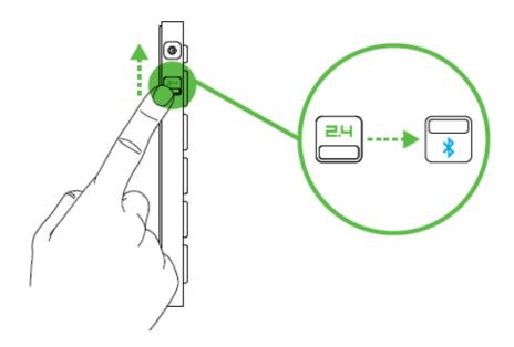
2. Press the Power button to turn the Razer Turret gaming lapboard on and activate pairing mode. The LED indicator will start to blink in blue.
