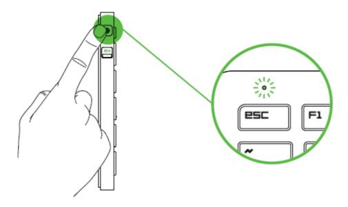
5. When successfully connected, the LED indicator will stay lit in green for 5s before fading off.
