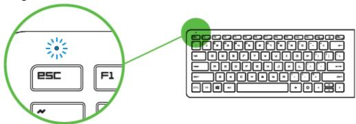
Note: To pair your Razer Turret gaming lapboard to a different device, disconnect the current Bluetooth connection from host device. Then, press and hold the power button for 3s to manually activate pairing mode.
