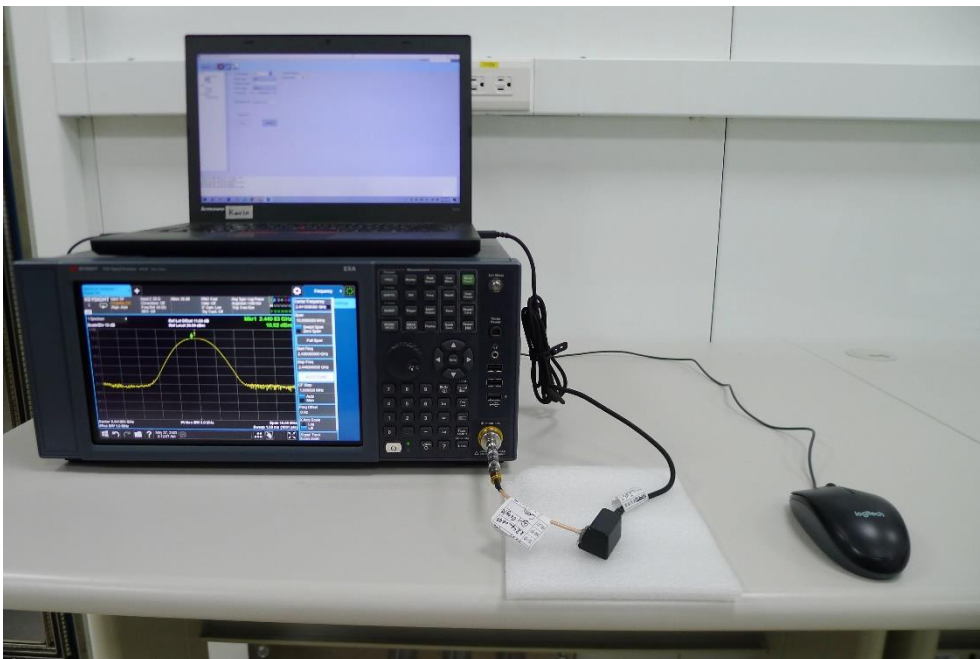
Description: Conducted Emission Test Setup
