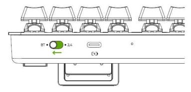
2. Up to 3 Bluetooth devices can be paired and registered to your keyboard (one for each profile). To activate the pairing mode of your preferred profile, press and hold its corresponding shortcut for 5 seconds. The LED indicators will then display which Profile has been activated.
