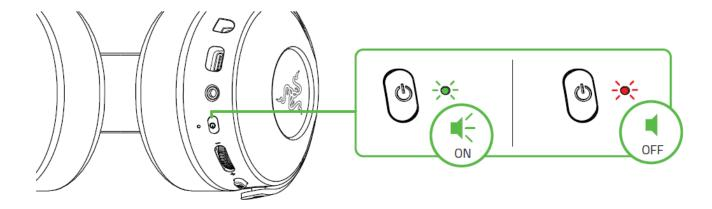
Other power button functions are available when the headset is powered on and connected to your device. These functions operate based on your device's current activity.
