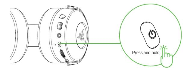
3. Wait until the status indicator briefly becomes static green indicating that the headset is now connected to the wireless USB dongle.
