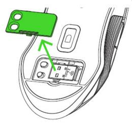
2. Remove the USB wireless receiver from the compartment and place it into PC's USB port.
