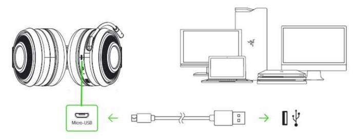
For best results, please fully charge your headset before using it for the first time. A depleted unit will fully charge in about **4 hours**.
