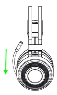
Bend the mic until it is parallel to your mouth, then adjust the length as preferred. Make sure the mic diaphragm is in front and the air vent is facing away from your mouth.
