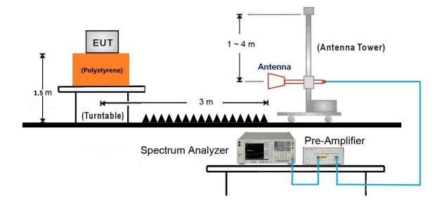
18GHz ~25GHz Test Setup:
