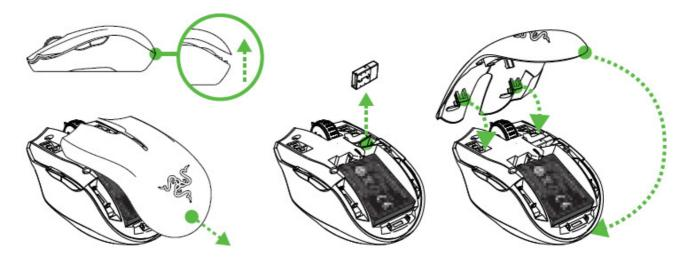
3. Plug the USB dongle to the device you wish to pair to.
