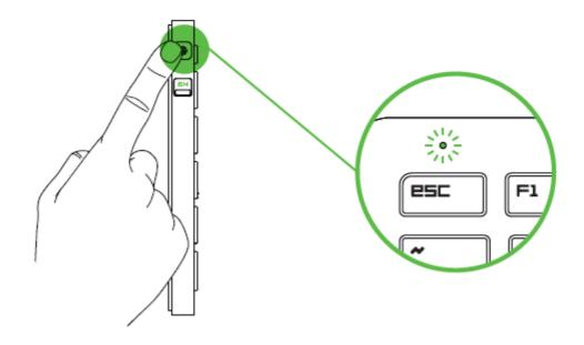
5. When successfully connected, the LED indicator will stay lit in green for 5s before fading off.
