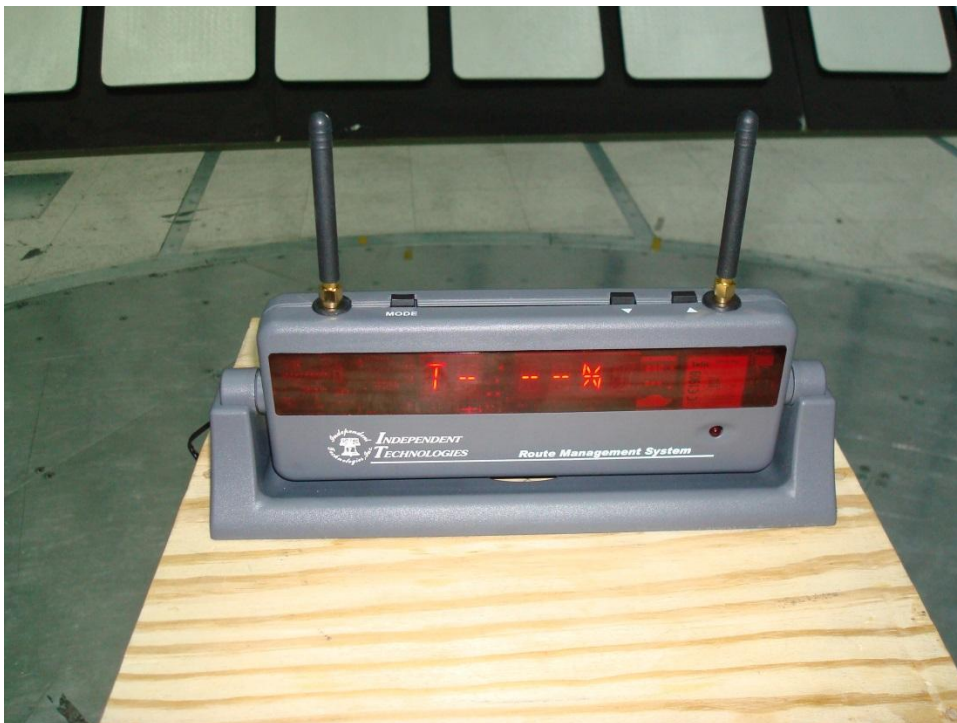
Figure 2 - Radiated Emissions Test Setup
