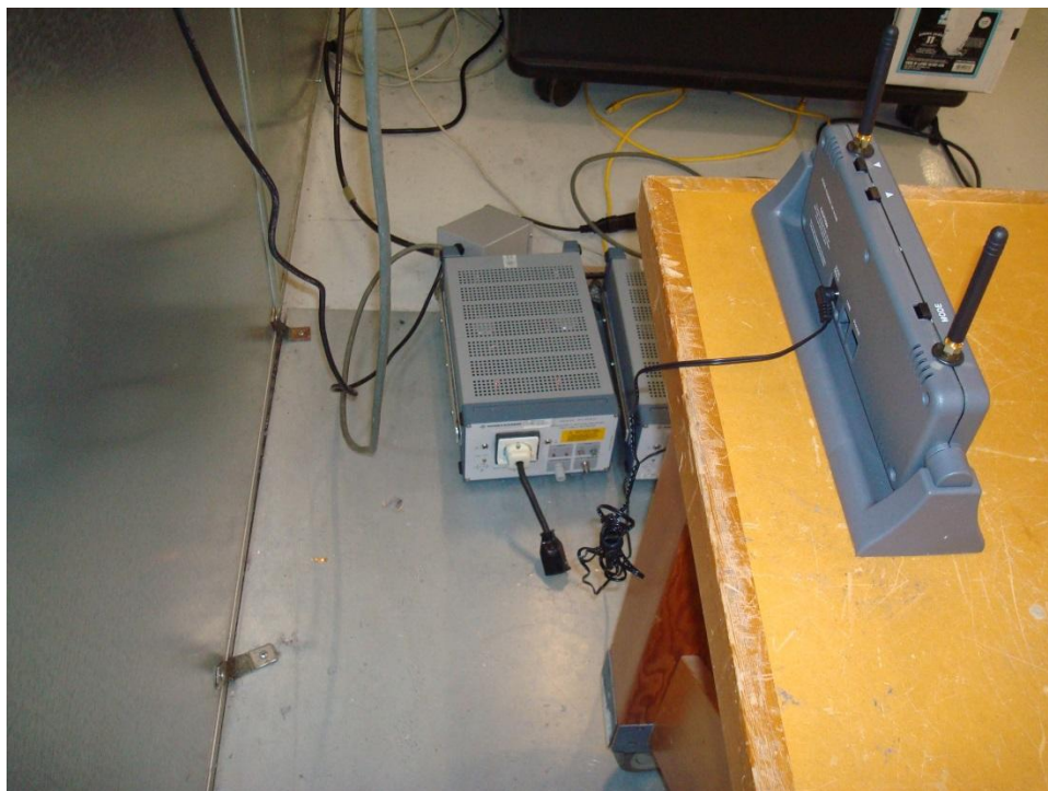
Figure 4 - Conducted Emissions Test Setup
