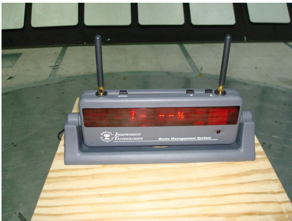
Figure 21 - Radiated Emissions Test Setup
