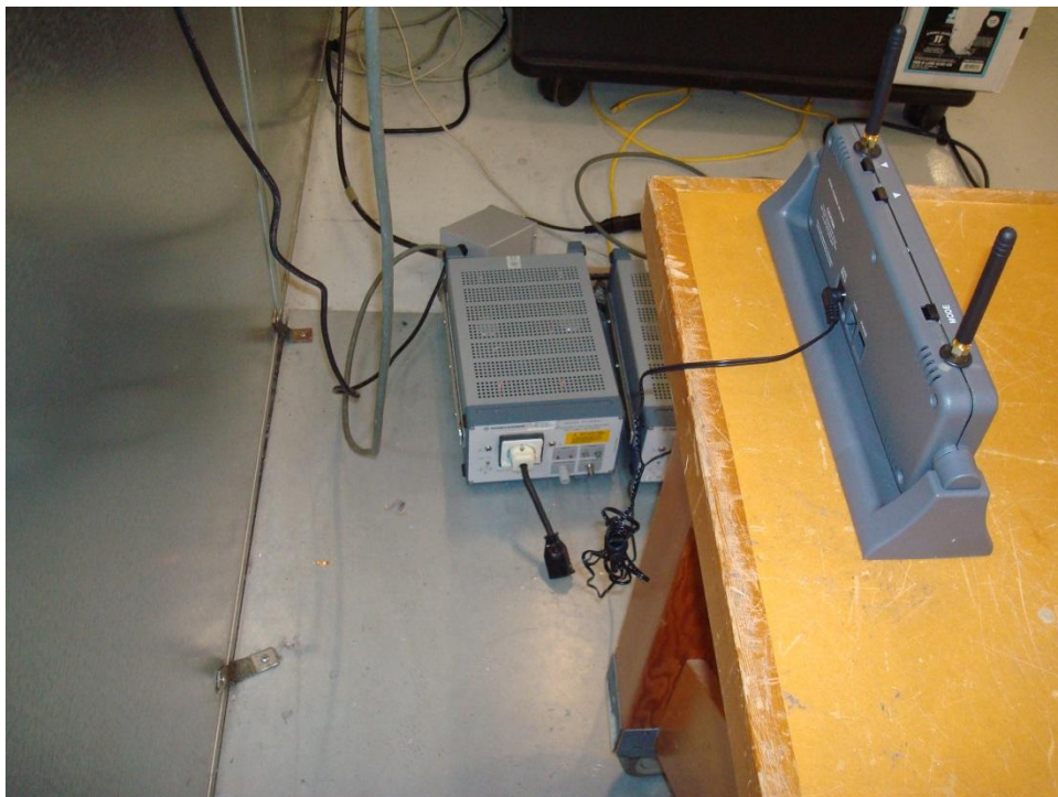
Figure 23 - Conducted Emissions Test Setup
