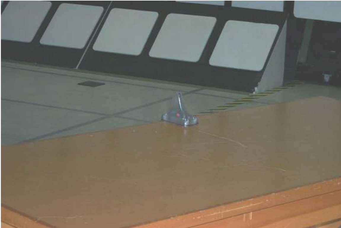
Figure 18 - Radiated Emissions Test Setup
