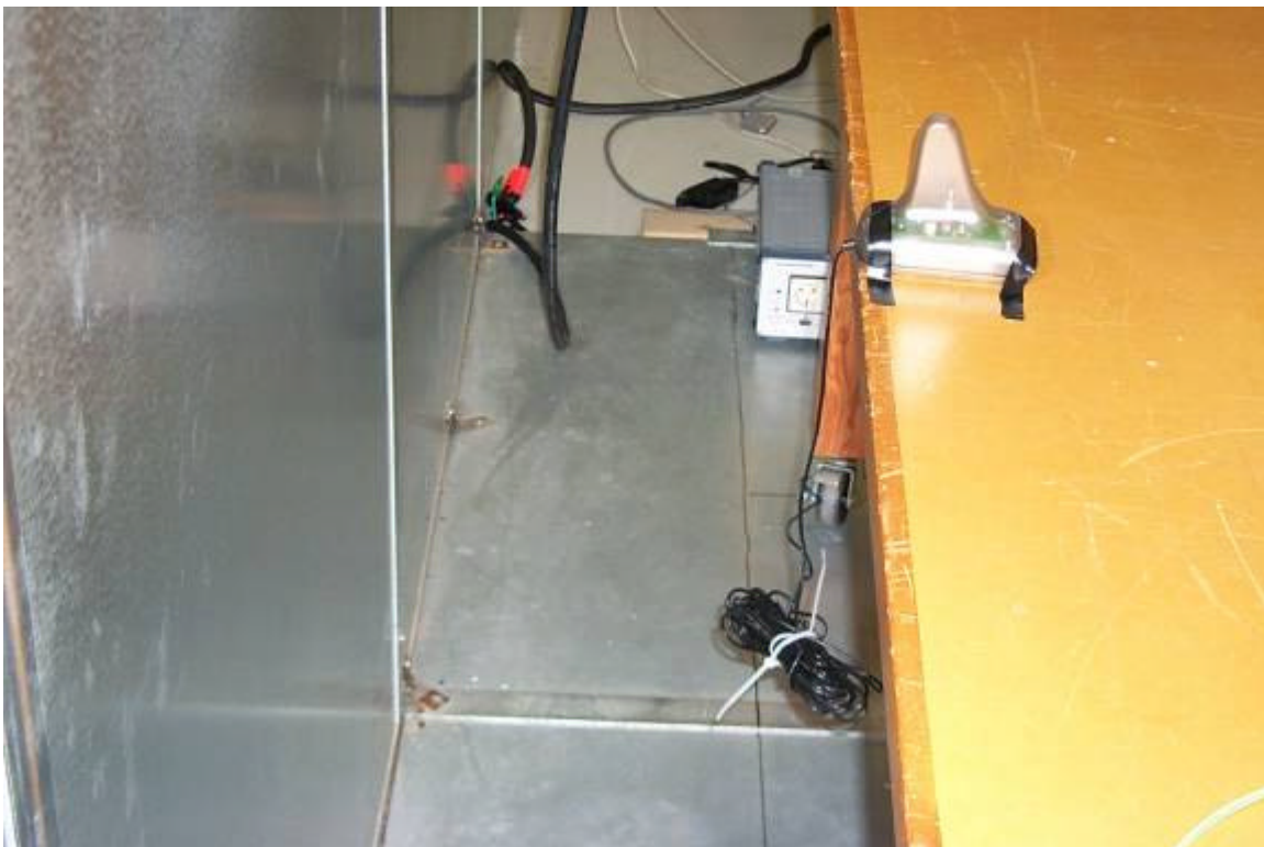
Figure 13 - Conducted Emissions Test Setup, MT-9100R-ACO
