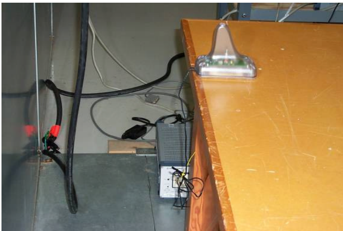
Figure 15 - Conducted Emissions Test Setup, MT-9100R-AC
