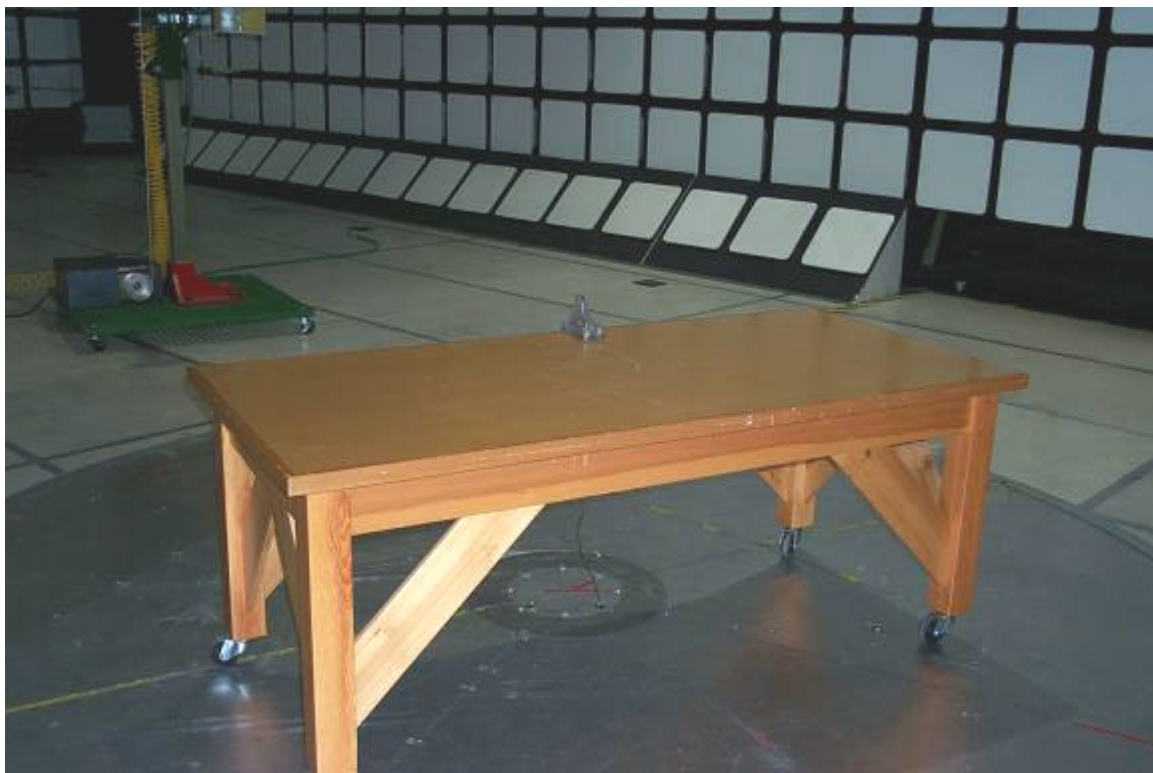
Figure 17 - Radiated Emissions Test Setup
