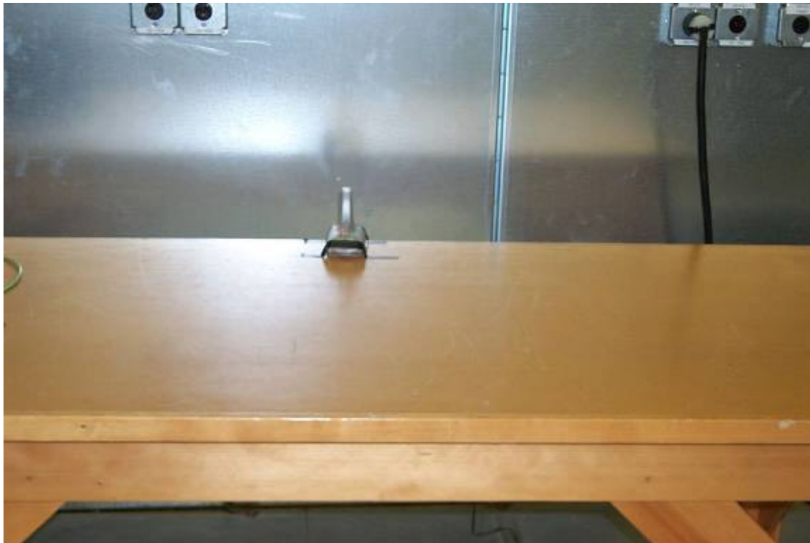
Figure 14 - Conducted Emissions Test Setup
