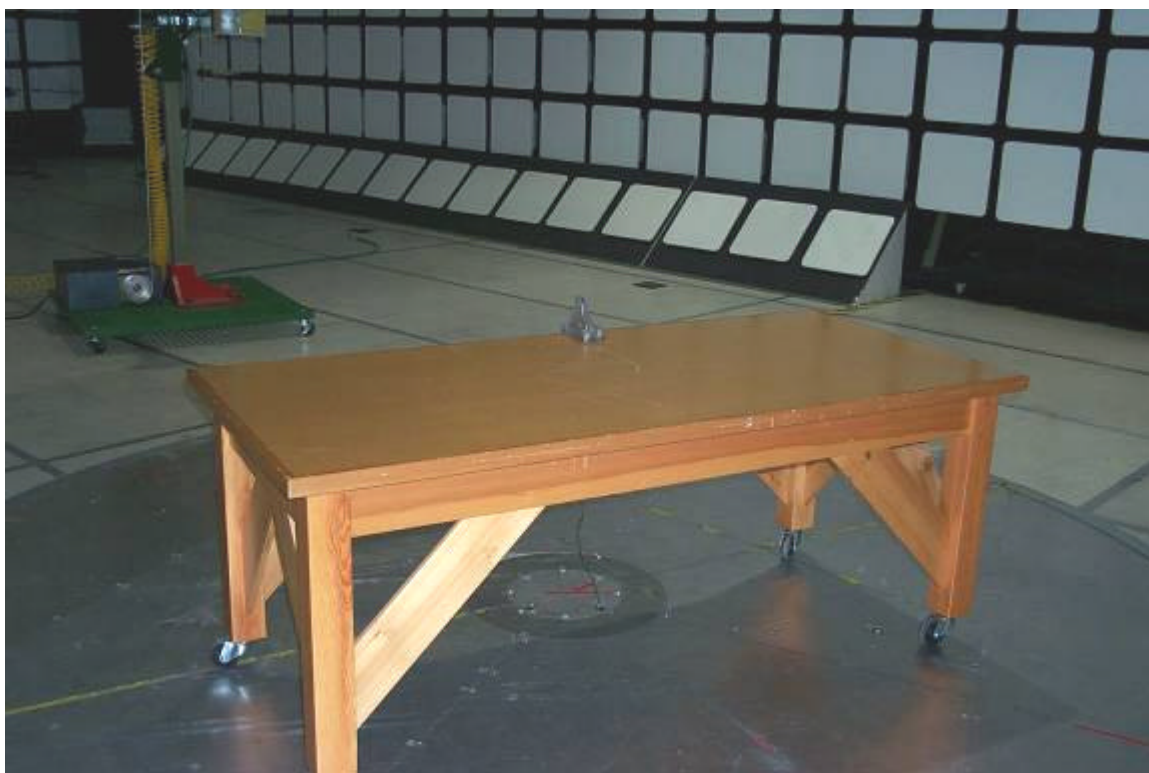
Figure 17 - Radiated Emissions Test Setup
