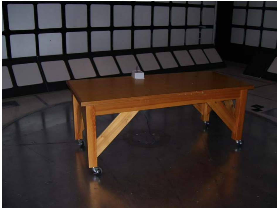
Figure 9 - Radiated Emissions Test Setup
