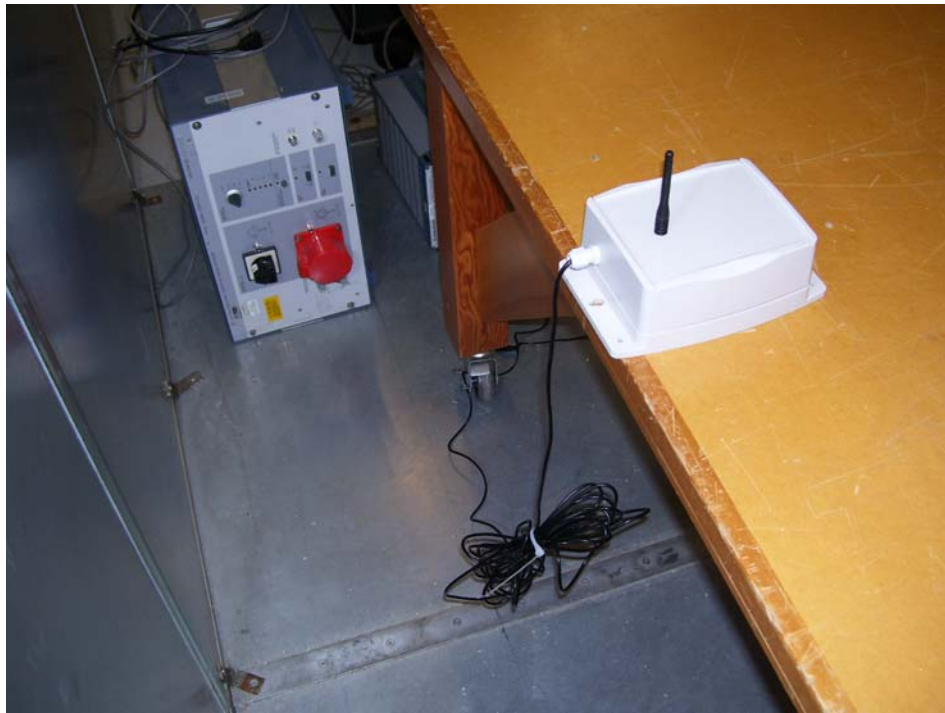
Figure 11 - Conducted Emissions Test Setup
