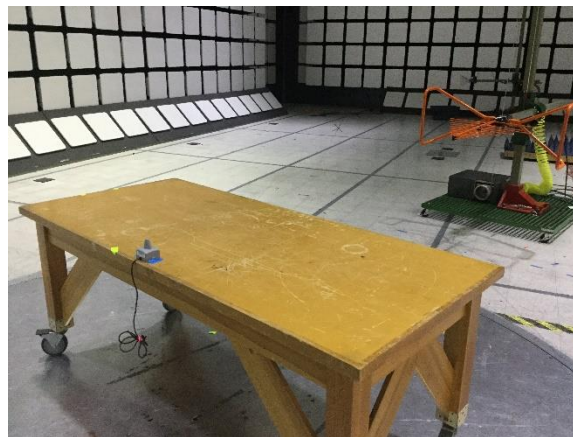
Figure 3 - Radiated Emissions Set up, Worst Case Orientation
