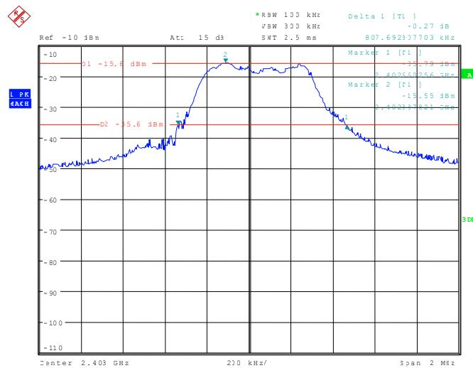
120019\_22.wmf: 20 dB bandwidth at the middle of the assigned frequency band:
