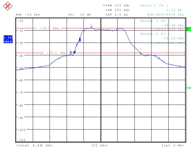
120019\_24.wmf: 20 dB bandwidth at the upper end of the assigned frequency band:
