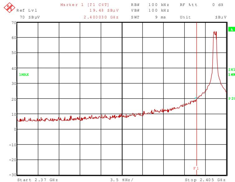
120019\_5.wmf: Radiated band-edge compliance, upper band edge (operation mode 3):
