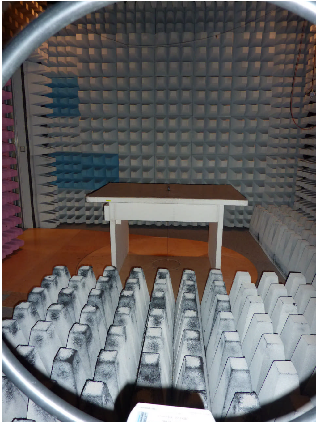
120019_6.JPG: RFS 2 transmitter, test set-up fully anechoic chamber
