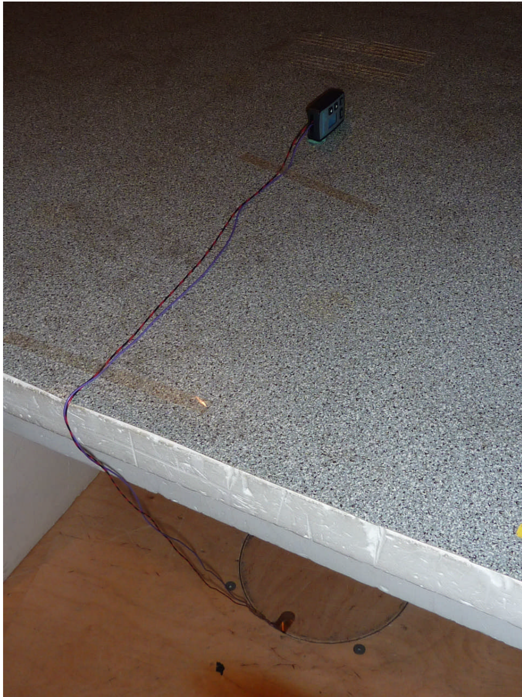
120019_2.JPG: RFS 2 transmitter, test set-up fully anechoic chamber (Pos. 2)
