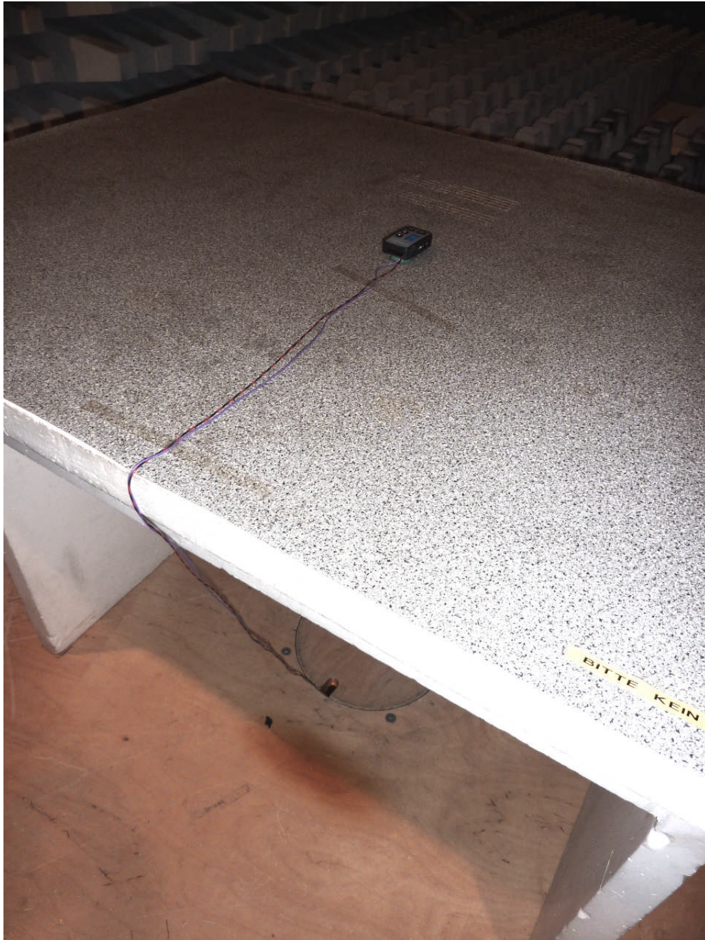
120019_3.JPG: RFS 2 transmitter, test set-up fully anechoic chamber (Pos. 1)
