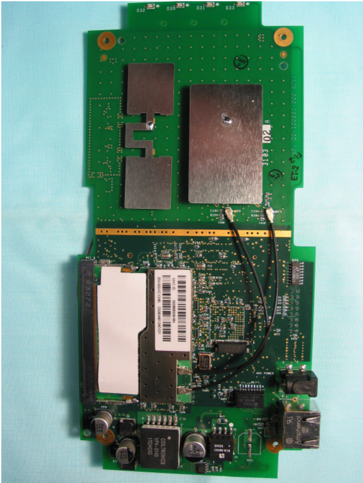
802.11 Access Point PCA, 802.11 BG side
