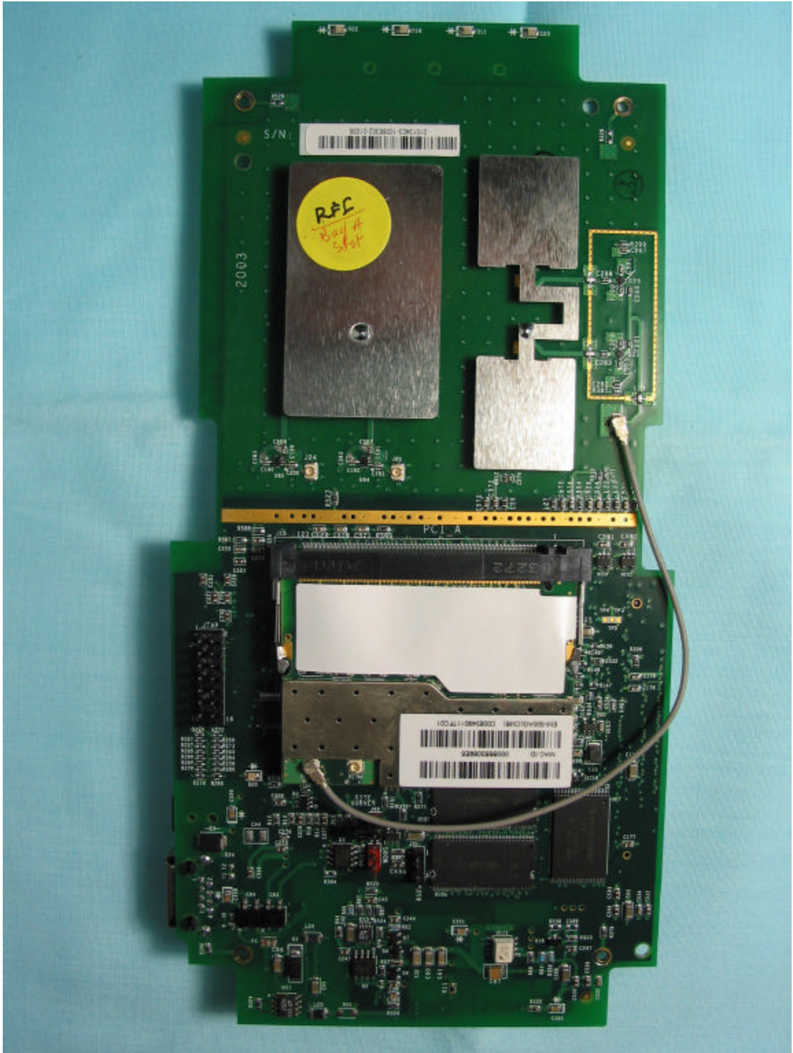
802.11 Access Point PCA, 802.11 A side
