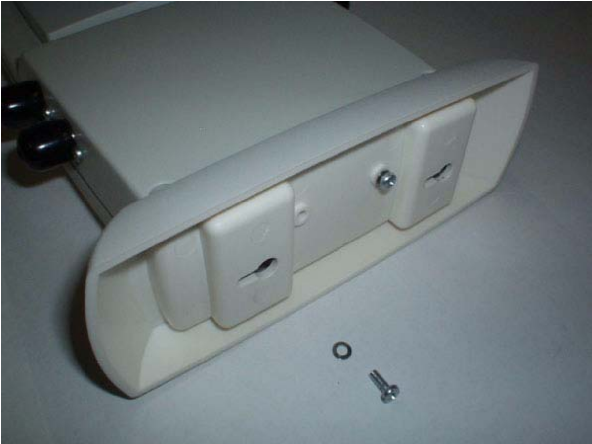
Figure - Assembling the Nortel Networks WLAN - Access Point and Ceiling-Mount Base
