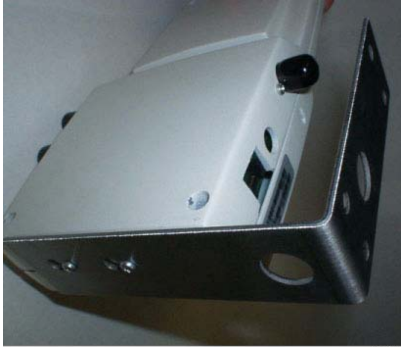
Figure - Assembling the Nortel Networks WLAN - Access Point to the Projection-Mount Bracket
