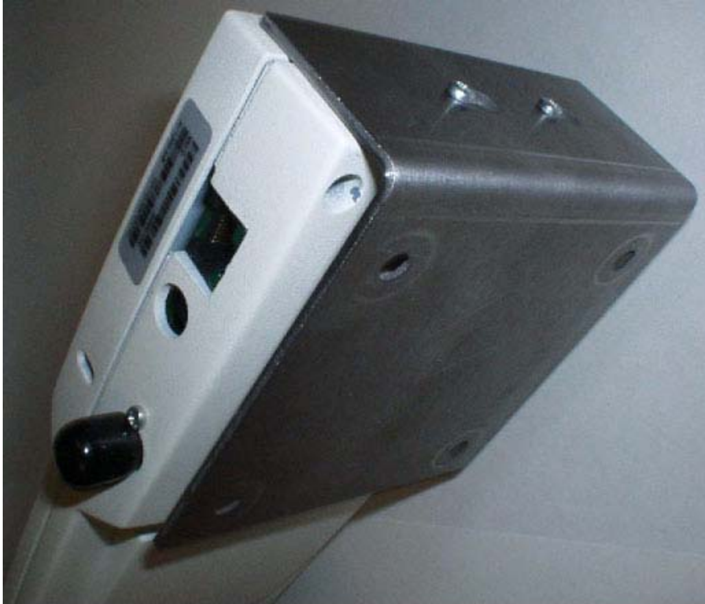
Figure - Assembling the Nortel Networks WLAN - Access Point to the Flush-Mount Bracket
