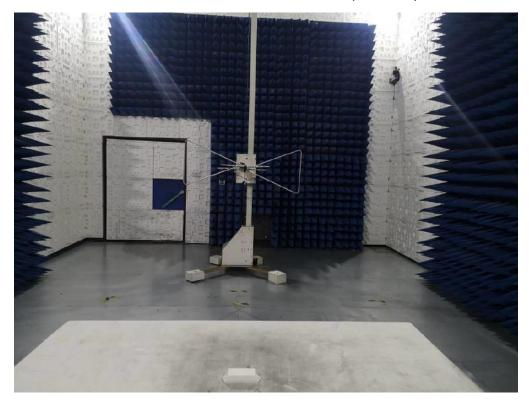
RADIATED EMISSION TEST SETUP (above 1G)
