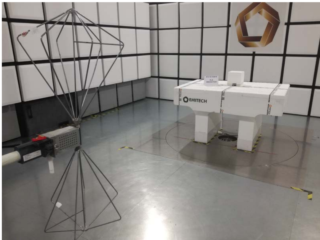
TEST SETUP PHOTO(S) – FOR 30MHZ <FREQ< 200MHZ
