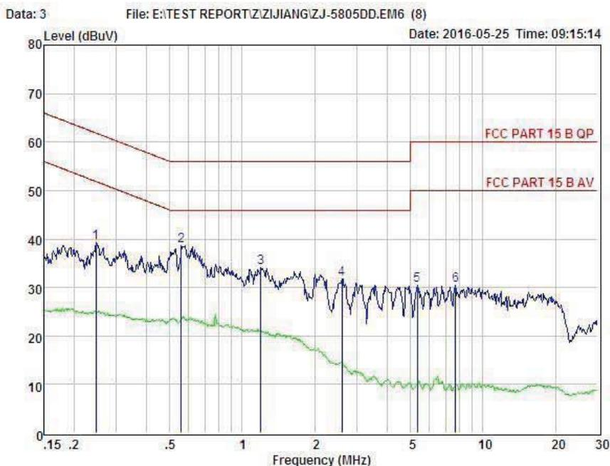
Condition : FCC PART 15 B QP POL: LINE Temp: 23.5 °C Hum: 54 %
