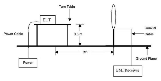
The diagram below shows the test setup that is utilized to make the measurements for emission from 30 Mz to 1  $\mathbb{G}_{\mathbb{Z}}$  Emissions.
