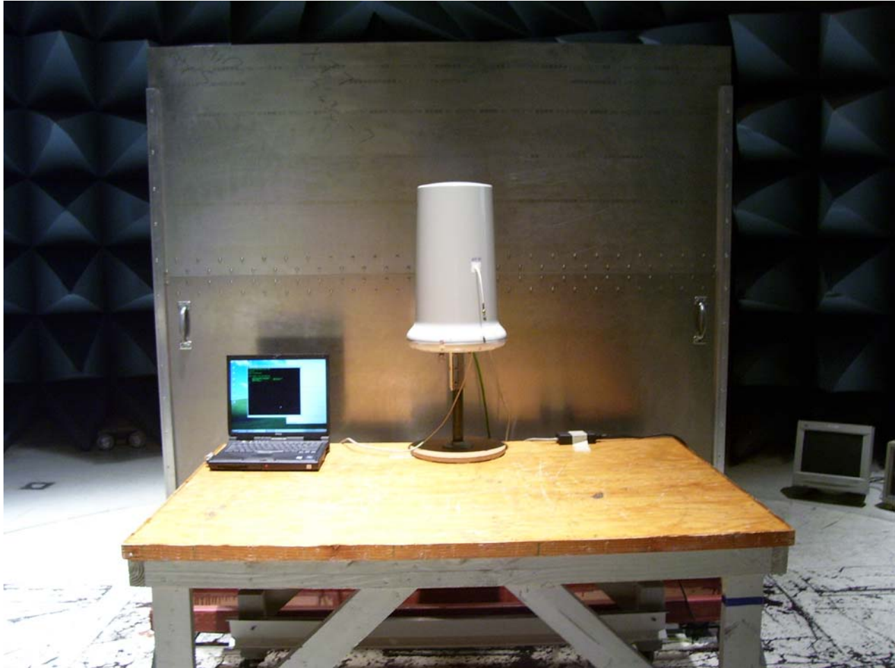
Conducted Emissions Test Setup
