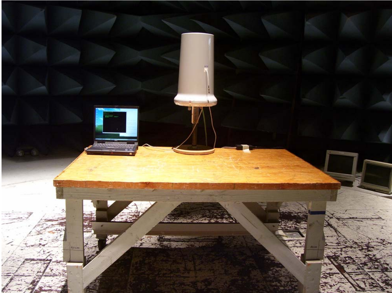
Radiated Emission Limits Test Setup
