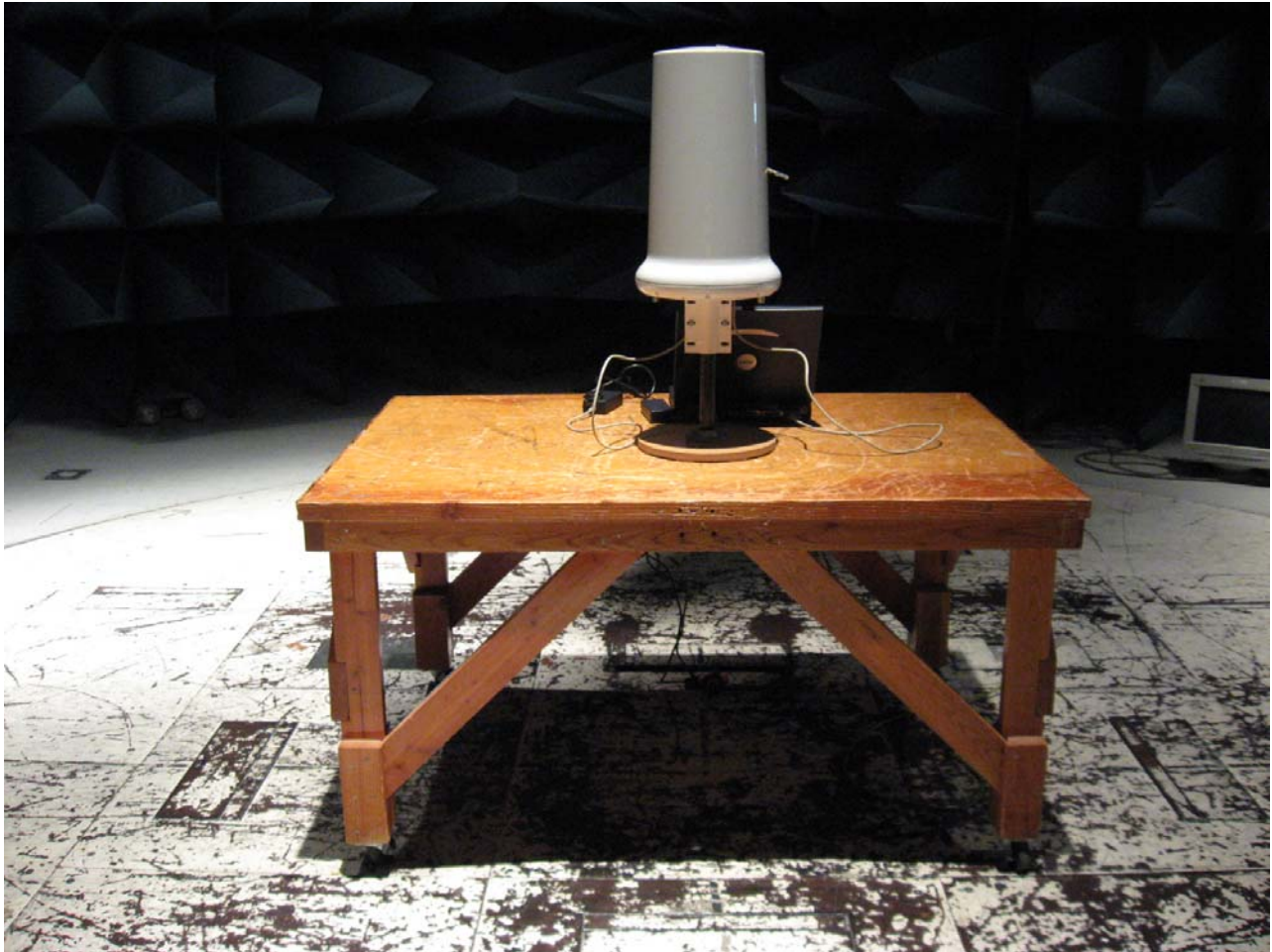
Radiated Emission Spurious Test Setup
