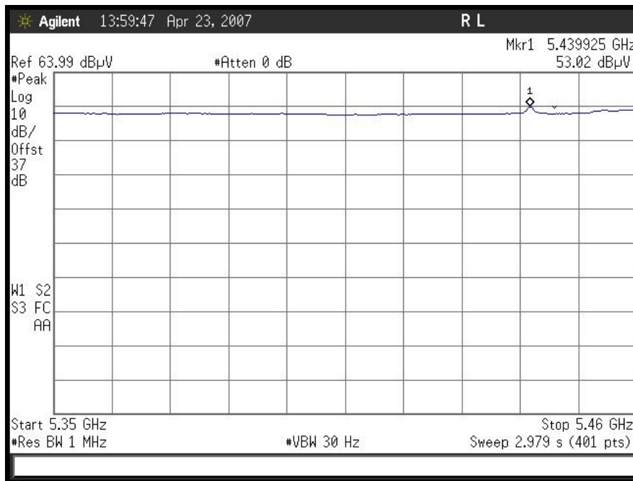
Plot 26. Restricted band (5350-5460MHz) with 5500MHz carrier-Average Measurement
