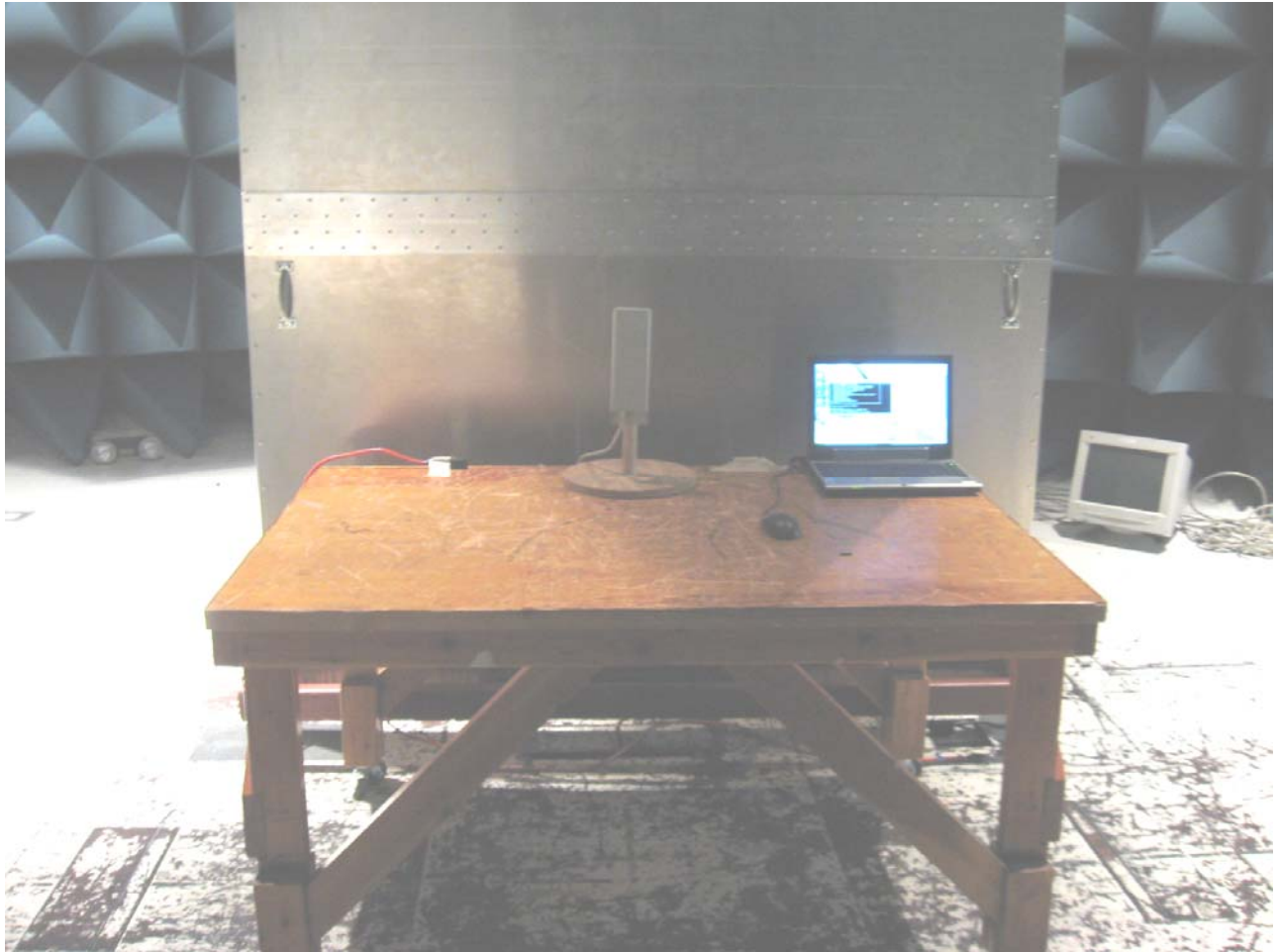
Photograph 4. Conducted Emissions Test Setup
