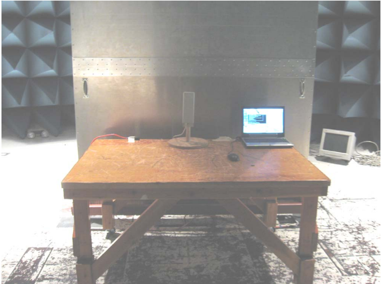
Photograph 2. Conducted Emissions Test Setup
