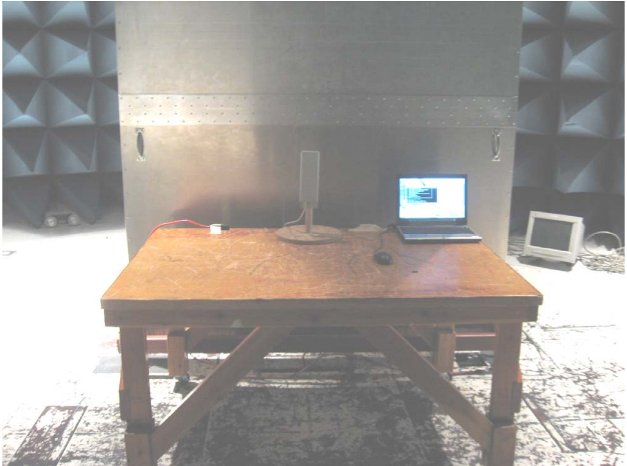
Photograph 2. Conducted Emissions Test Setup
