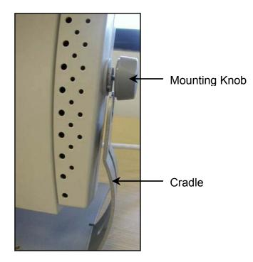
If there is no suitable flat surface, then the user should install the window mounting bracket. This can be installed on a window ledge or on the side or top of a window frame. The CPE is then attached to the bracket via one of the supplied mounting knobs. Note that the CPE must always be mounted vertically.
