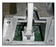
The gasket is then placed around the cable.
