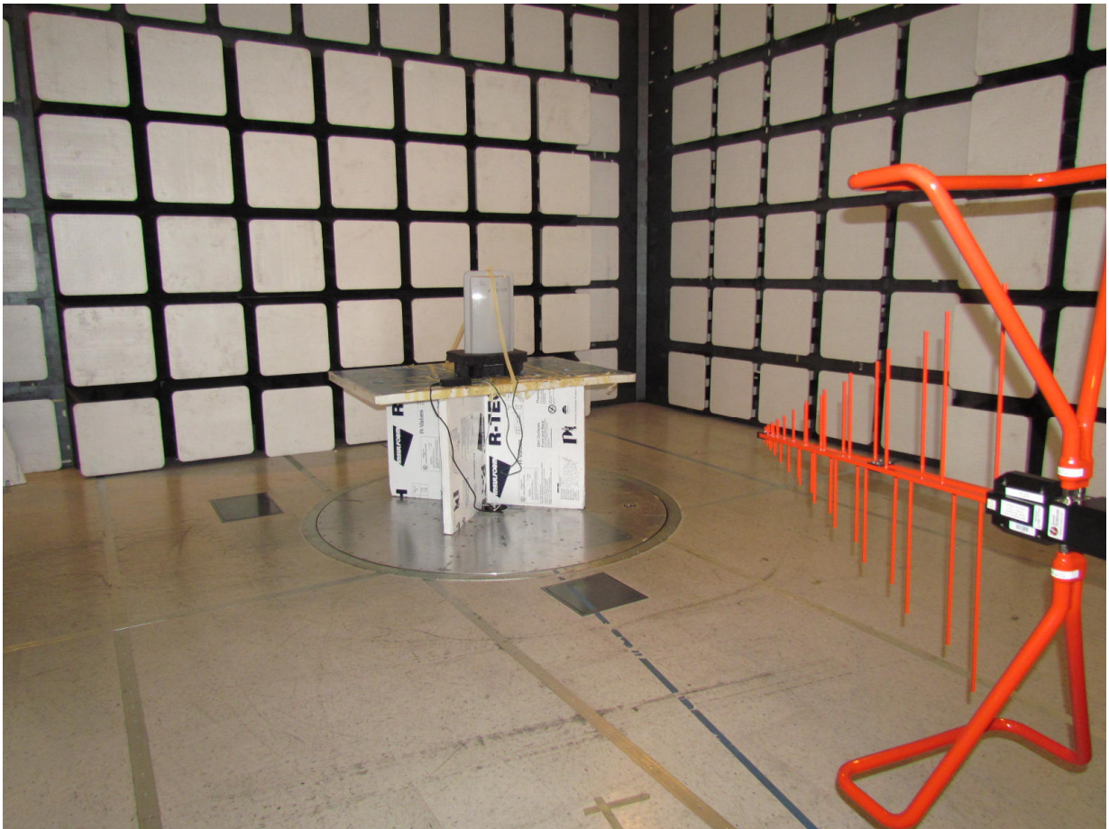
Radiated Emissions Below 1 GHz - Test Setup
