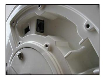
In order to ensure full weatherproofing, the grommet provided must be installed. The Ethernet cable should first be connected and then pushed into the slit in the gasket and then the gasket is pushed into the opening in the base. See the photograph below.
