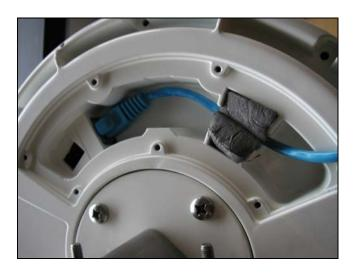
Finally the cover is installed using the provided screws. The Ethernet cable is position to pass through the insert in the cover. It is highly recommended that the cover and gasket be fitted in a Seed Only application (i.e. no subscriber or WAN interface).
