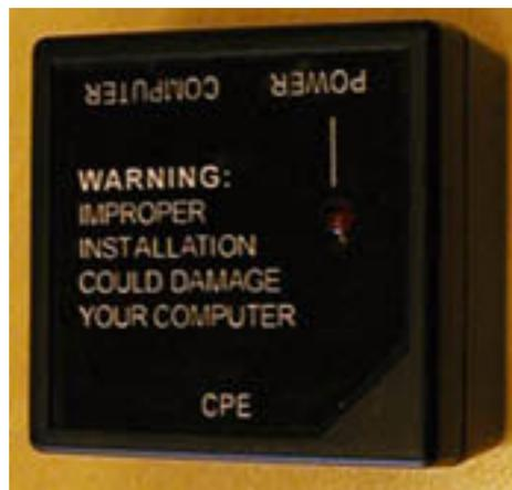
Figure 2-2 Power Injector
