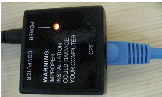
Figure 2-10 Connection To Power Injector
