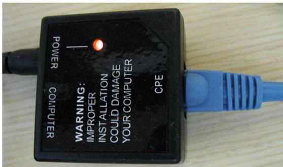
Figure 2-14 Connect To Power Injector
