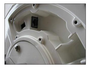
In order to ensure full weatherproofing, the grommet provided must be installed. The Ethernet cable should first be connected and then pushed into the slit in the gasket and then the gasket is pushed into the opening in the base. See the photograph below.
