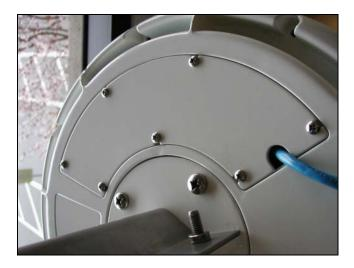
Once the node is installed, it is recommended that the Ethernet cable be secured to prevent strain (particularly installations exposed to high wind conditions). The photograph below shows an example were the cable is secured to the mounting pole.
