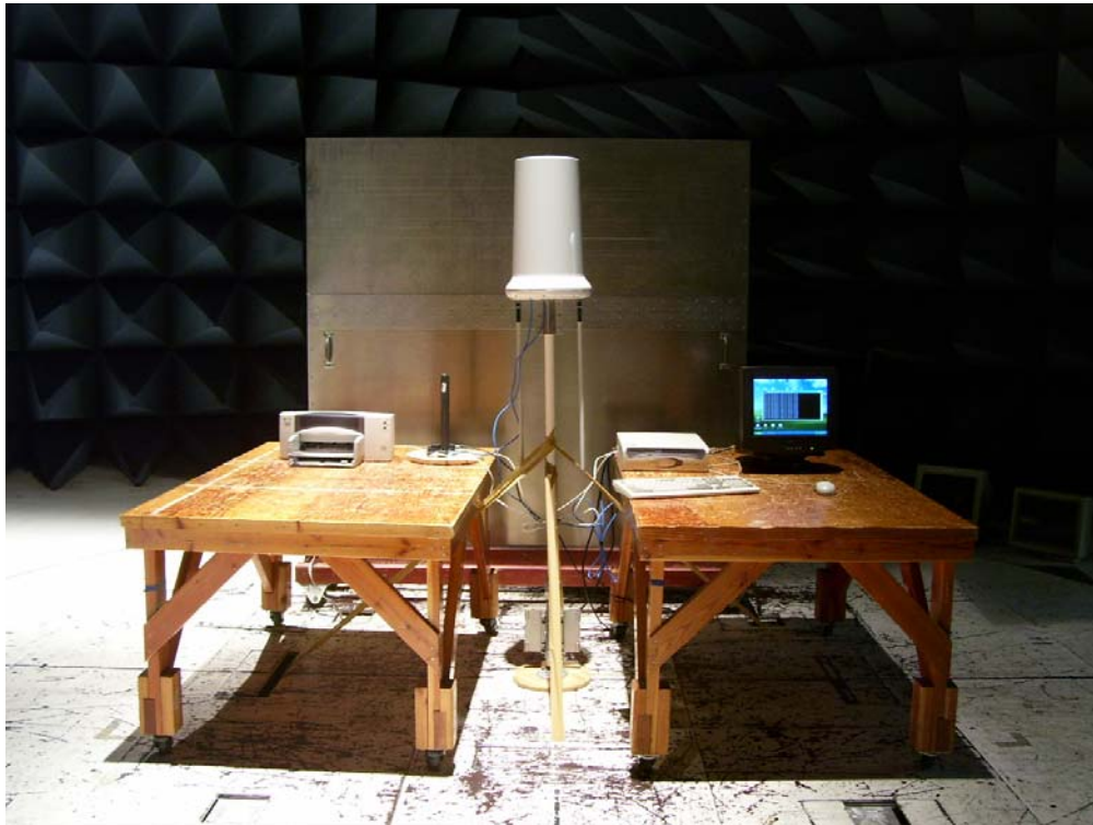
Photograph 3. Conducted Emissions Test Setup
