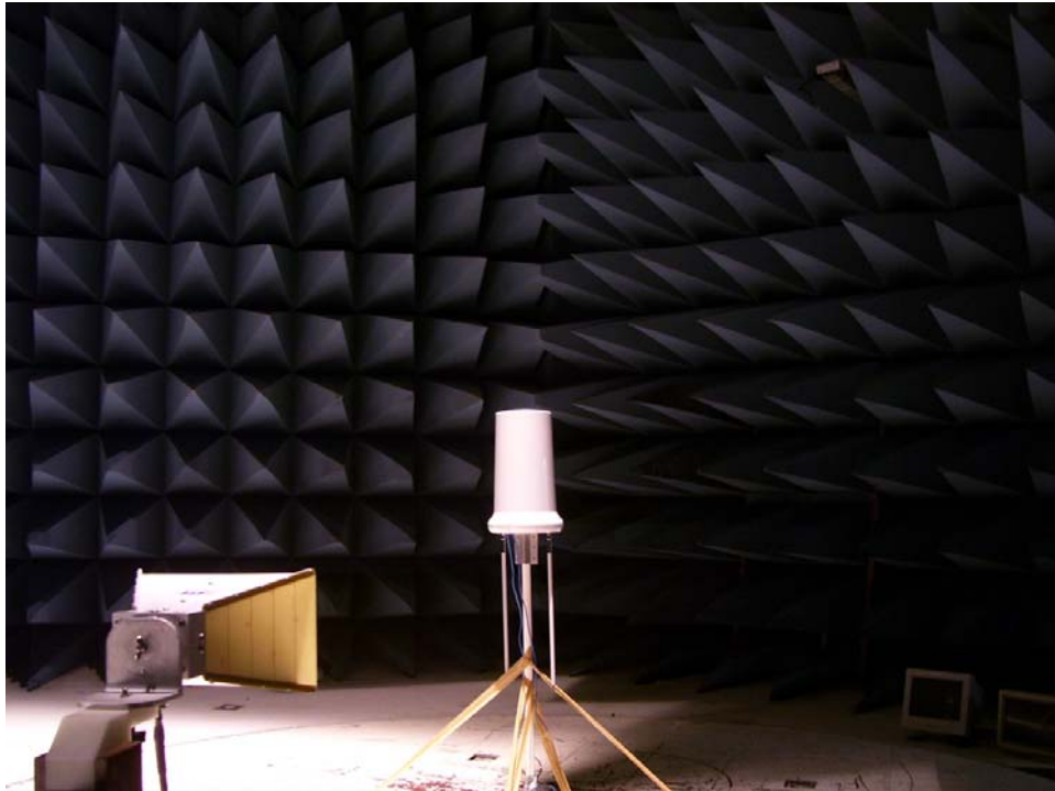
Photograph 2. Radiated Emission Spurious Test Setup
