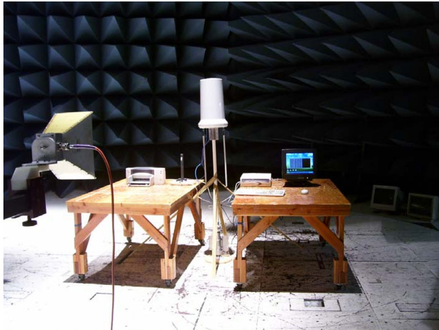
Photograph 7. Radiated Emission Limits Test Setup for 1-2GHz
