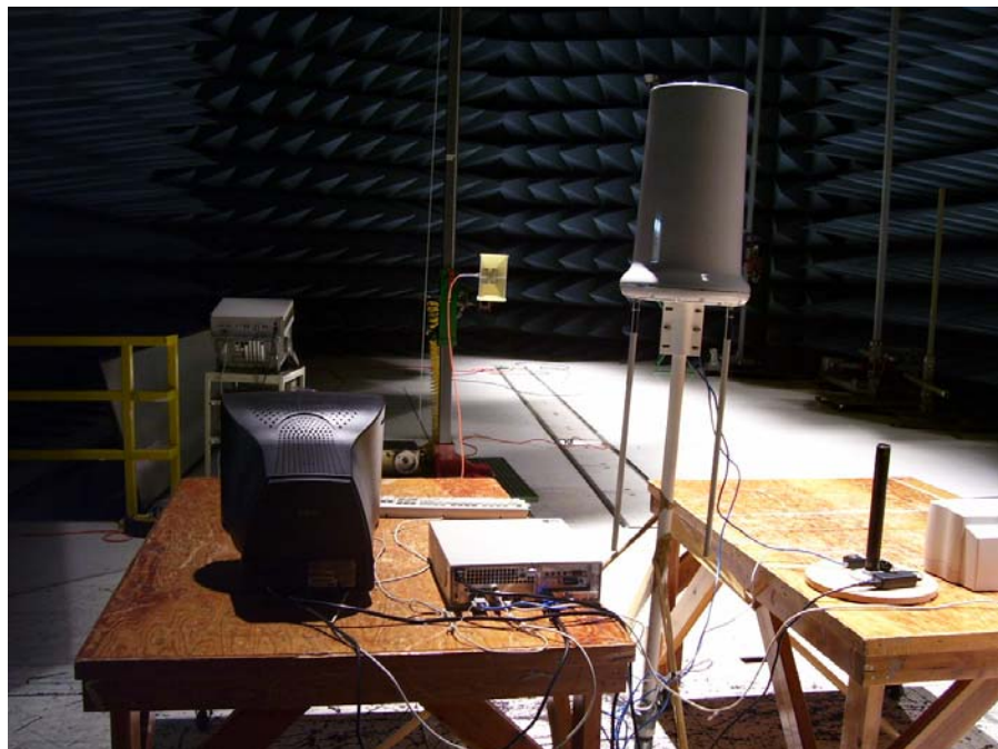
Photograph 8. Radiated Emission Limits Test Setup for 1-2GHz
