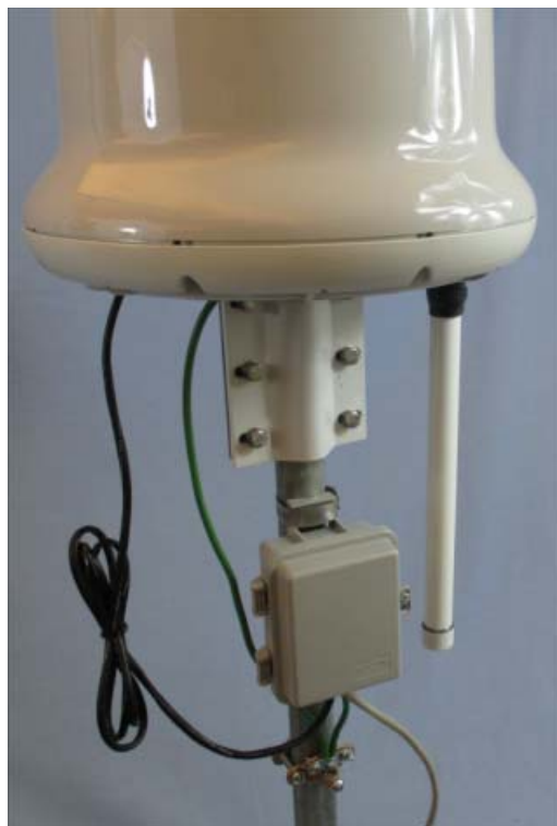
Figure 1 Assembled and installed Extender Bridge with Citel surge suppressor
