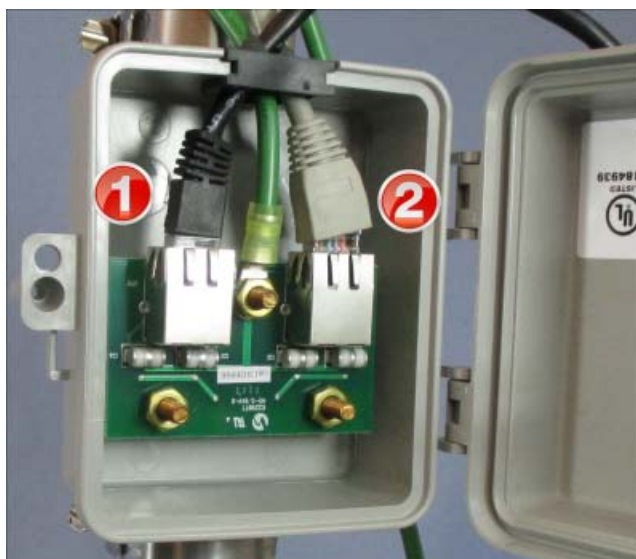
Figure 7 Citel surge suppressor with gasket and cables
