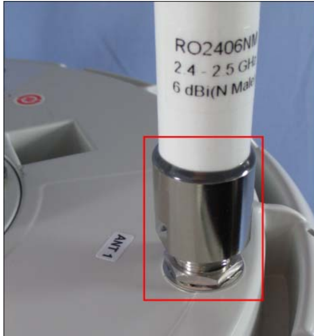
Figure 26 NAN Antenna mounted on base
