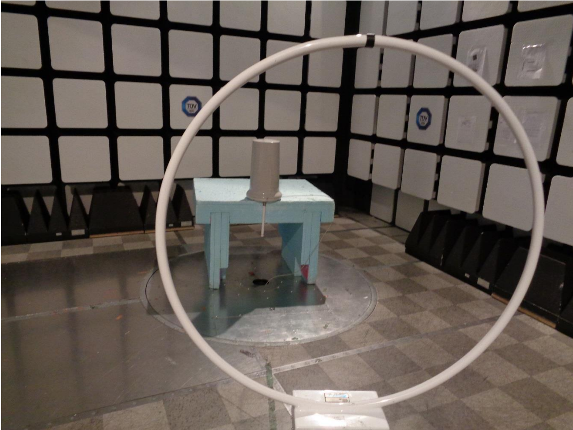
Figure 2 – Radiated Emissions Setup 9kHz – 30MHz
