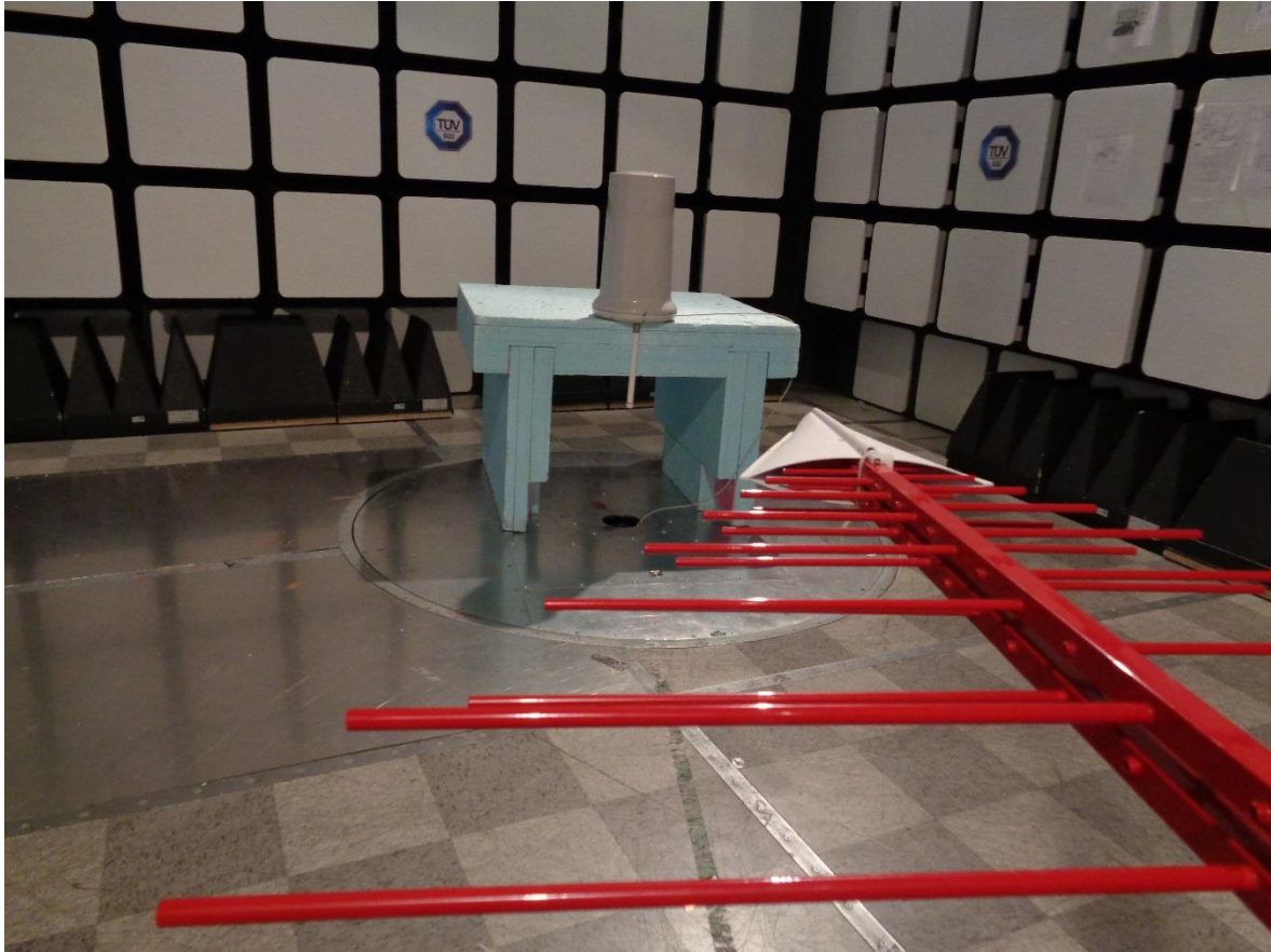
Figure 3 – Radiated Emissions Setup 30MHz – 1GHz
