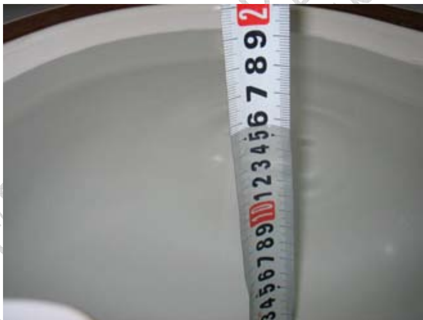
Picture 10 Liquid Depth at Ear Reference Point for 1900MHz Head Liquid
