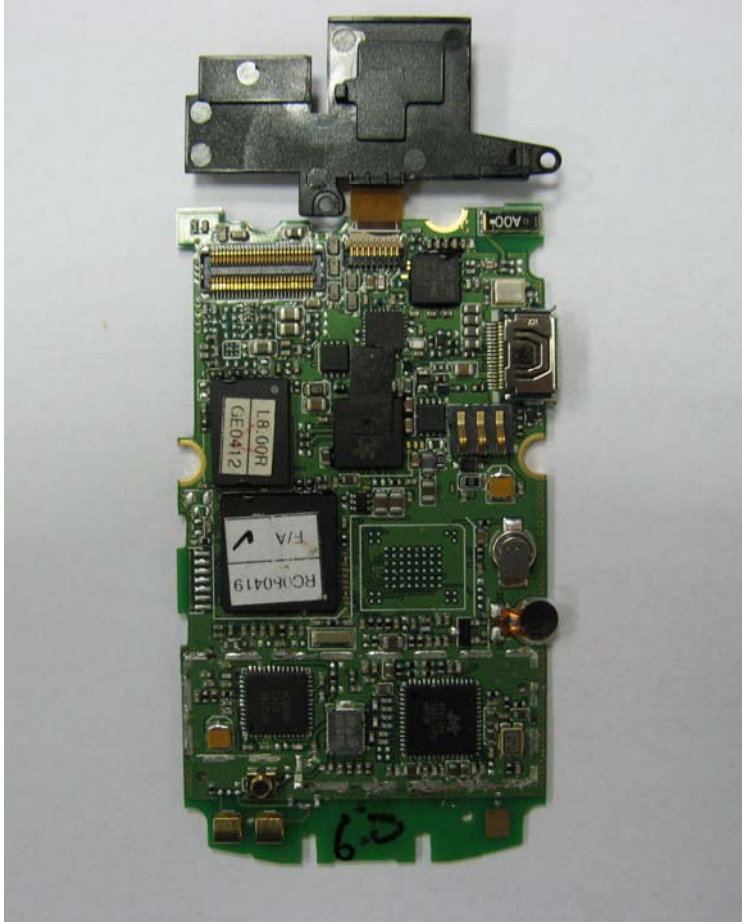
Picture 3: The sample with the shielding cover removed
