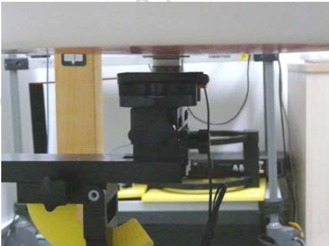
Picture 8 Body SAR Front to the phantom, with headset
