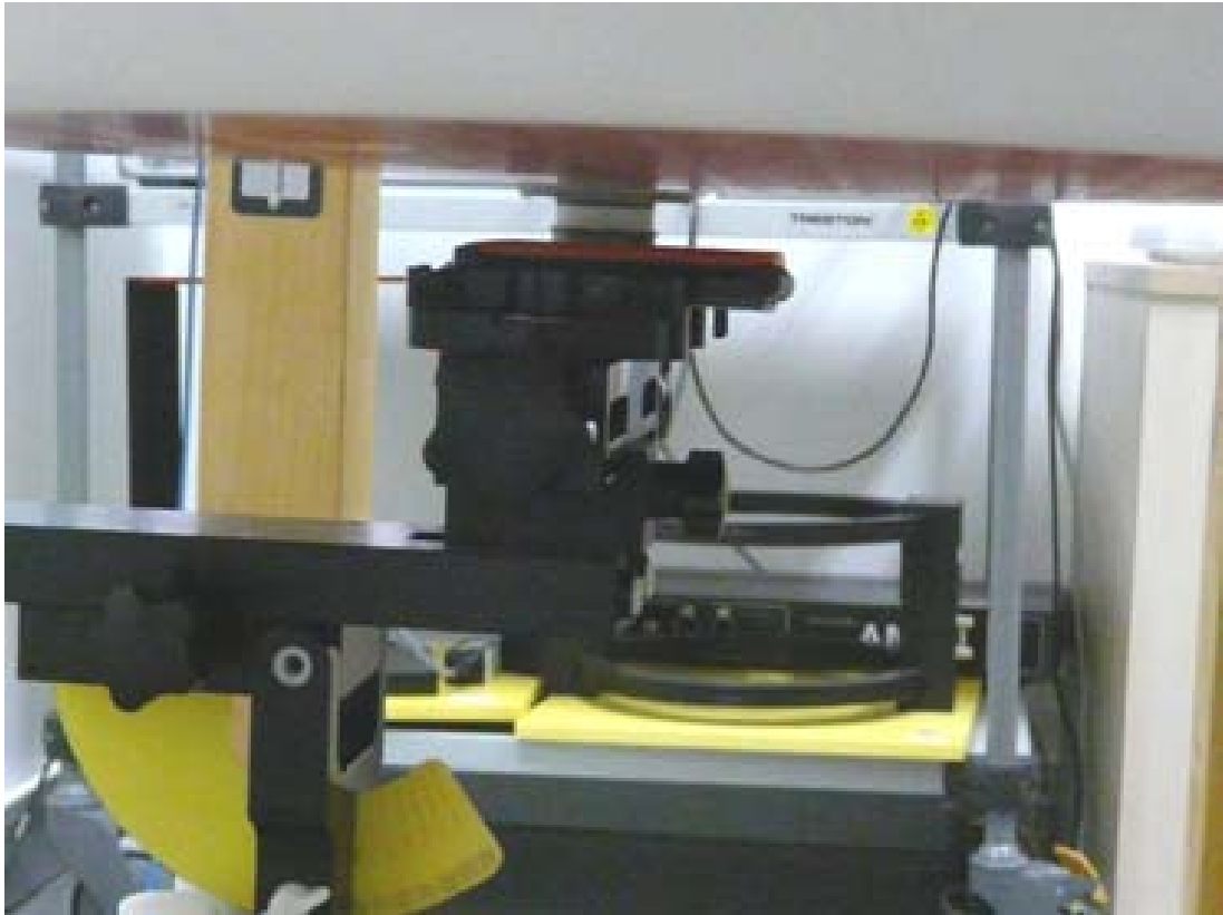
Picture 7 Body SAR Front to the phantom
